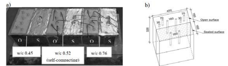
Fig. 1. (a) Concrete samples. O = open surface, S = sealed surfaces; (b) Schematic drawing of measuring boreholes in open surface sample.
